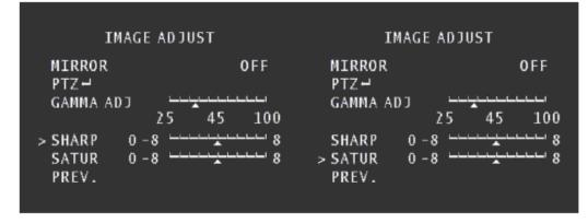
**SHARP:** The overall image sharpness can be adjusted to soften or crispen the image. Making the image crisper can produce higher resolution images, but noise becomes apparent. Default is 0.
