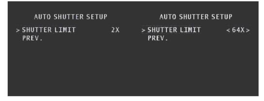
**AUTO:** The camera uses a combination. of applied gain and slow shutter to compensate for decreased light levels. If select the "SLOW SHUTTER" mode, shutter speed limit can be set. Shutter speed limits:X2,X4,X8,X16, X32, X64 optional. The default is X2
