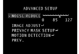
NOISE REDUCE: Noise Level can be adjusted from 0-127 to remove image noise. ADVANCED SETUP - IMAGE ADJUST
