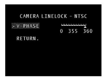
**V-PHASE:** Allows the user to adjust the vertical phase of the output video when SYNC is set to Line-Lock.
