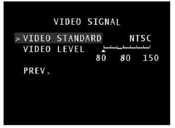
VIDEO STANDARD: PAL/NTSC selector. Changes NTSC video or PAL video system for camera.
