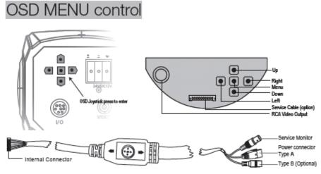
The Menu can be either buttons or joystick control. Pressing the middle button will activate the OSD menu options Service cable (optional) on some models.
