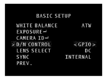
**AUTO:** The system gain, set manually or automatically computed by the exposure subsystem, will be used to determine whether the camera should be in day or night mode. Night mode will be entered when the system gain is above a threshold. If the gain falls bellow this value the mode will change to day mode. Sub-menu allows the threshold to be set.
